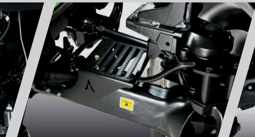
> Maintenance steps above the front axle for comfortable cleaning.
