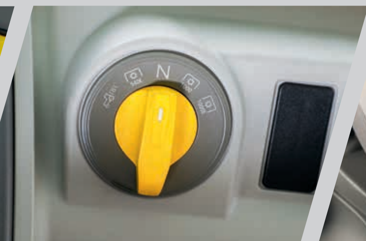
> Electrohydraulic PTO selection.
