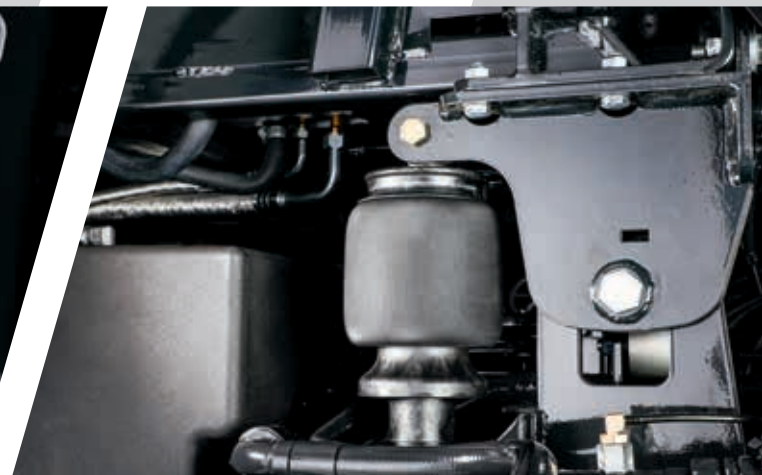
> Pneumatic cab suspension for a smoother ride.
