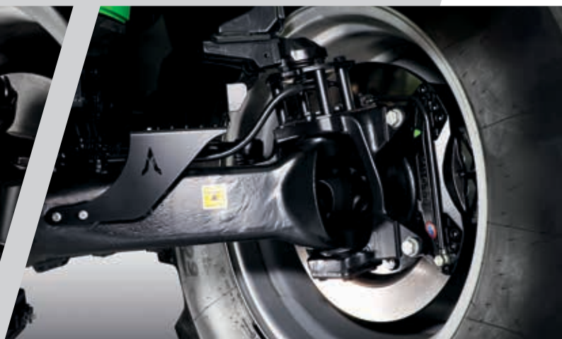
> Dry disc brakes for maximum brake performance.
