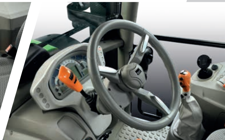
> PowerShuttle with SenseClutch 5-levels adjustment and Stop&Go function.
